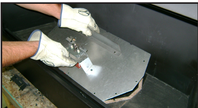
Figure 11.3. Remove Valve Plate
